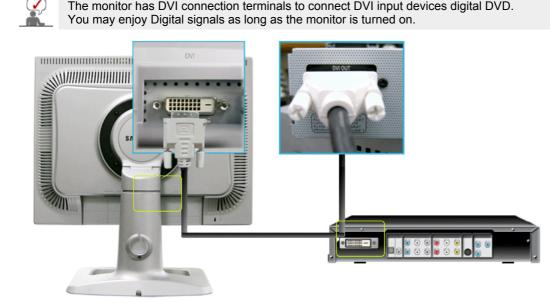
1. Input devices such as digital DVD is connected to the DVI terminal of the monitor using the DVI cable.
